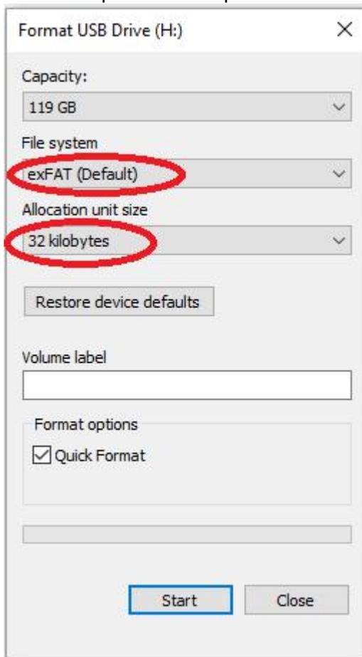
**PS:** Switch doesn't support exFAT by default. Before next step, please put micro SD card inside switch SD card slot. System will prompt to update system patch after power on. You can connect to internet to update exFAT support. Offline update exFAT support is possible, please Google "How to install the exFat Update without updating your Switch".
