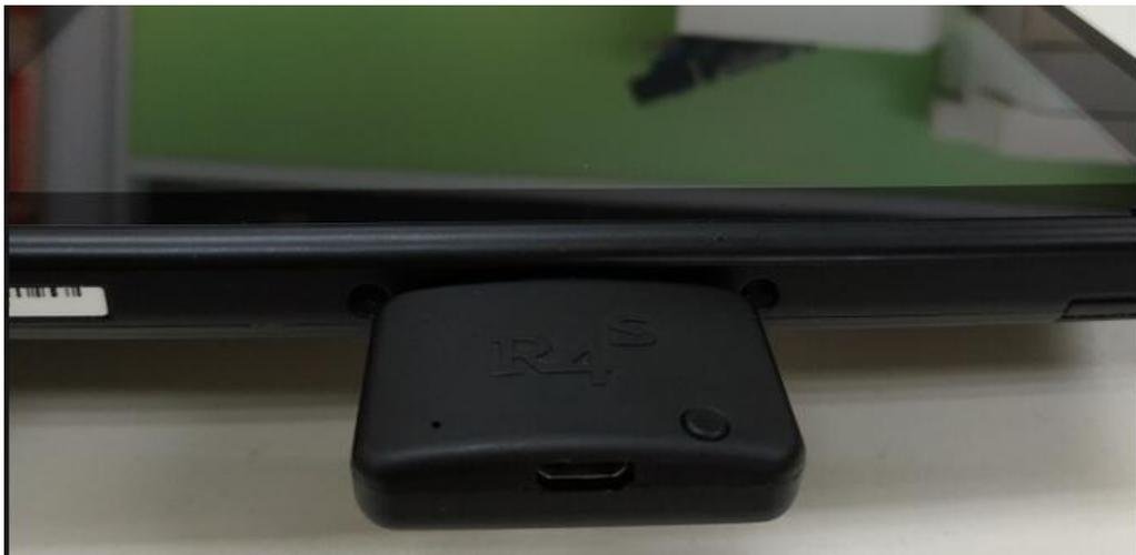
4. Hold the VOL + button and power button to turn on the Switch, the red led on the dongle will be light, and the system should boot into the customer firmware.
