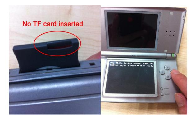
7. Repairing program start, makes sure NDSL console has enough power, and do not remove the flash cart during repairing process.
