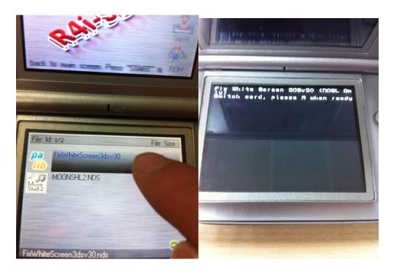
6. Do not shut down the power of the console. Replace the working flash cart with the problem r4i-sdhc white screen flash cart. Then press button "A" to start repairing. Attention: Do not insert micro SD card to the problem r4i-sdhc white screen flash cart during upgrading.
